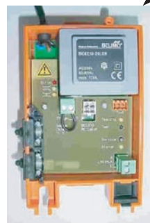
Communication and power supply unit BKN230-24LON (LonMark certified)
